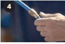
**4** Slide the lower portion of the FastFix Fitting past where the hose is damaged
