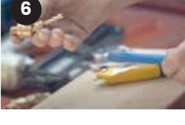
**6** Remove the barbed swivel fitting from the end of the hose
