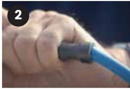
**2** Pull the bend restrictor past where the hose is damaged
