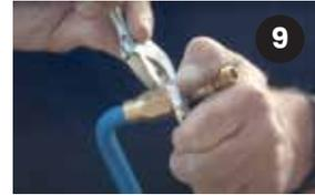
Slide the bend restrictor back up to the fitting
