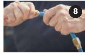
Slide the lower part of the Fastfix fitting and screw onto the swivel and tighten
